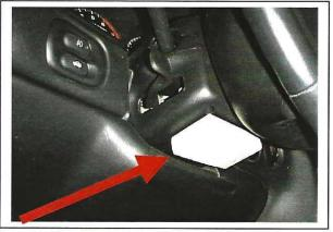
Someone on one the 'Vette bulletin boards suggested using double sided tape and attaching the garage door opener to the flat space under the steering wheel. I thought that was entirely too easy, ain't no power tools needed, but I checked anyway. Shazzam, it works GREAT. It is very accessible and is not in the way, in fact it is not visible at all. No more digging to find the opener. A very simple and cheap fix. I attached a picture to show where it goes. Happy Motoring!
