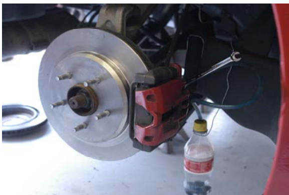
New rotor on and now draining old fluid out!
